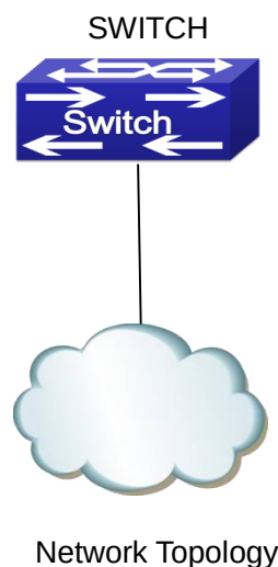
Figure 2-3 Typical example of port loopback detection
